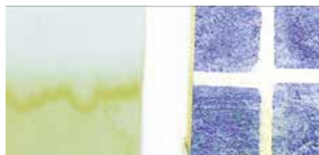
Liners that have come in contact with sun cream and chlorinated water that contains copper.
