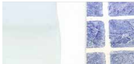
Liners that have come in contact with sun cream and chlorinated water.
