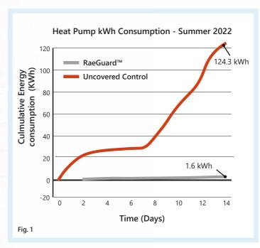
RaeGuard™ offers up to 90% of the insulating performance of a traditional 5mm foam, but with a significant reduction in the material cost.
