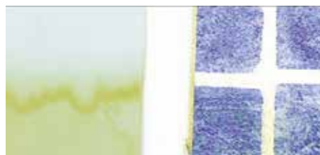
Liners that have come in contact with sun cream and chlorinated water that contains copper.
